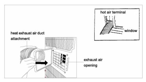
Correct mounting shown below (if mounting in the wall, the height of the hole should be 16" – 51")
